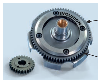
202.1222 Vespa 125 ET3 Z=27/69 Primary ratio-Primario
