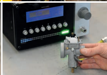
NEEDLE SEAL CHECK CONTROLLO TENUTA SPILLO
