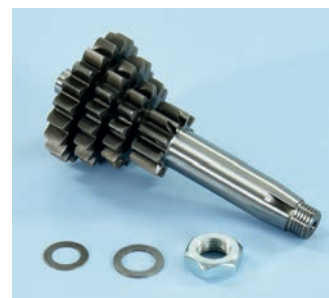
202.1417 Vespa 50/125 ET3 Z=10-14-17-20 Primary ratio-Primario
