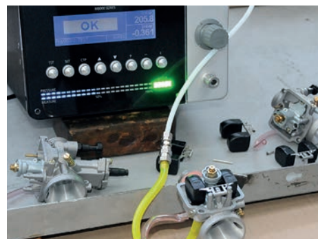
NEEDLE SEAL CHECK CONTROLLO TENUTA SPILLO
