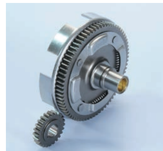
202.1217 Vespa 125, ET3,PK,ETS Z=27/69 Primary ratio-Primario
