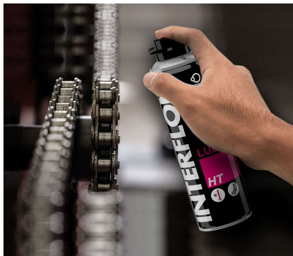
Oven chains can be lubricated with a heat-resistant chain oil, such as Interflon Lube HT
